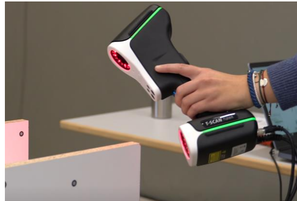
Figure 4: Hand held 3D scanner which was used to capture deviations
